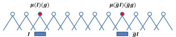
Fig. 8: Covariance: the response for an image I at position g is equal to the response of the group shifted image at the shifted position.
