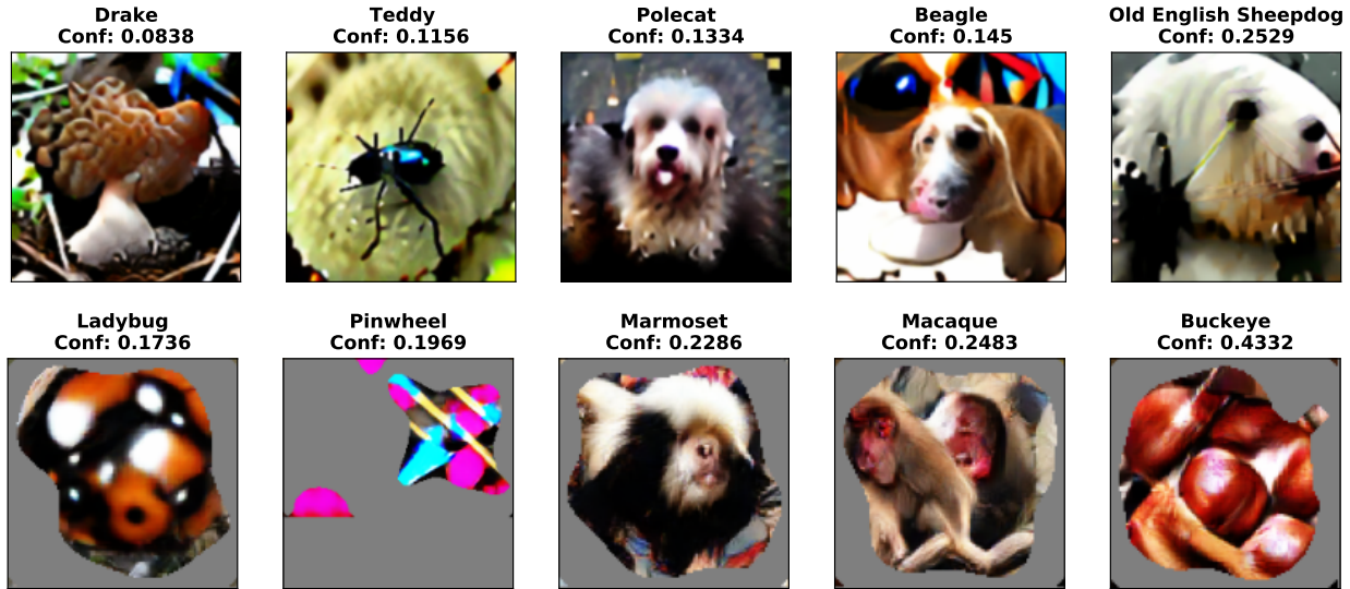
Figure 9. Black-box adversarial patches (top) and generalized patches (bottom) created using transfer from an ensemble. Patches are displayed alongside their target class and mean fooling confidence.
