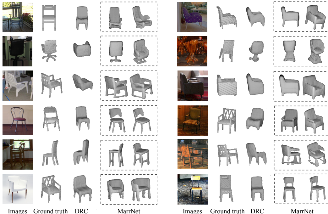
Figure 6: 3D reconstructions of chairs on the Pascal 3D+ [Xiang et al., 2014] dataset. From left to right: input, the ground truth shape from the dataset, 3D estimation by DRC [Tulsiani et al., 2017], and two views of MarrNet predictions. Our model recovers more accurate 3D shapes.
