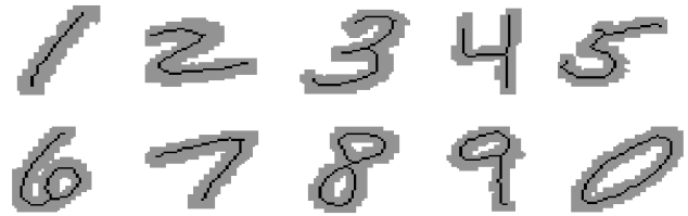
Figure 3. Symmetry axis being applied to hand-written digits 0-9.
