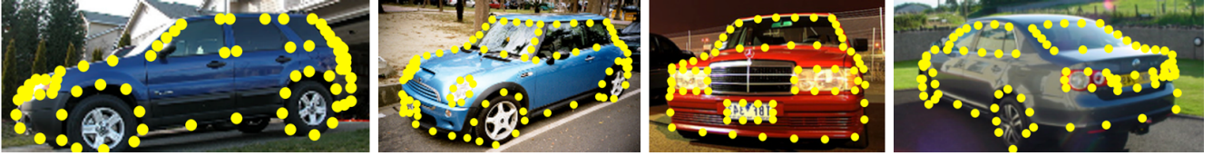
Figure 5: The landmark annotations for typical images. Yellow dots are the chosen landmark locations. Please refer to Section 3.3 for landmark selection criteria.
