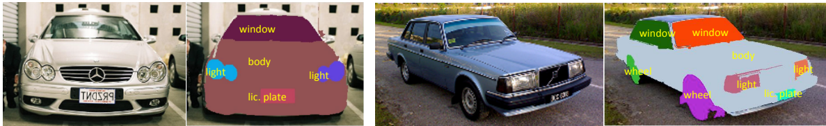
Figure 1: The goal of car parsing is to detect the locations of semantic parts and to perform object part segmentation. The inputs (left) are images of a car taken from different viewpoints. The outputs (right) are the locations of the car parts – the wheels, lights, windows, license plates and bodies – so that each pixel within the car is assigned to a part.
