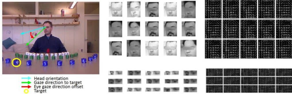
Figure 2: Computational appearance-based model. (Left) In each of the gaze trials the Appear-Face-Eyes model associates the face with the head pose orientation (cyan), and the eyes appearance with the eye-gaze correction offset (red). The ground truth gaze direction (green) is the direction from the center of the eyes towards the target (yellow). (Middle) Extracted nearest neighbors for both face and eyes during a query event. Each neighbor is associated with an orientation, and the final direction is determined as the weighted average of these orientations, where the weights correspond to the neighbors’ similarity with the query appearance. (Left) Rendered images of the Histogram of Gradients (HoG) descriptors used to represent face and eyes appearance. These robust general purpose image descriptors capture both edge and texture properties and allow spatial tolerance.
