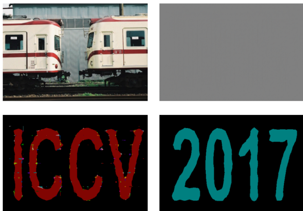
Figure 8: Figure taken from Xie et al. (2017). The top row is the input (adversarial perturbation already added) to the segmentation network, and the bottom row is the output. The red, blue and black regions are predicted as airplane , bus and background , respectively.
