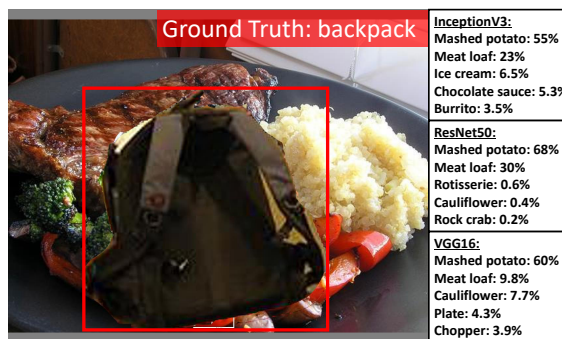
Figure 1. Mis-classification of objects in unfamiliar contexts. State-of-the-art deep visual recognition networks, such as InceptionV3 [42], ResNet50 [53] and VGG16 [40], make mistakes when the context is incongruent. The top-5 labels and confidence levels by each model are shown on the right.
